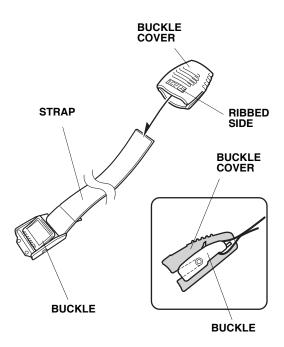
Route the strap under the front crossbar, and around the kayak as shown. Slide the buckle cover away from the buckle, route the strap through the buckle, and tighten the strap. Slide the buckle cover back over the buckle.
